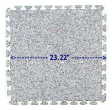
ElectraLock is a unique, 3 mm thick, precision cut ESD Control Vinyl Tile. ElectraLock features a diamond hard wear resistant top surface bonded to a full surface electrically conductive bottom layer, thus providing ultimate static control properties. ElectraLock is fully compliant to the latest ANSI ESD S20.20-2021 standards.
