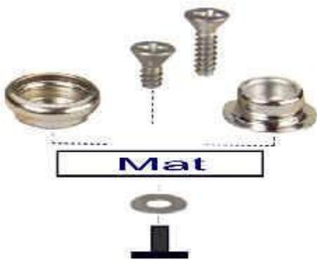
**INSTALLATION OF SNAP KIT (included with your order):** Push the base thru one of the 2 pre drilled holes located on the corners of the mat (use the small washer if needed for a tight fit). Place the male fastener on top of the mat and (using the small screw) tighten the assembly with a screw driver.
