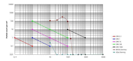
Representation of the relative success of cleaning the test area correlated to Surface Cleanliness Classes in accordance with VDI 2083 Part 9.1
